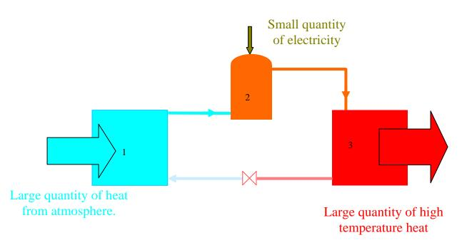
Energy is extracted from the air or from water condensing out of the air onto the evaporator.
