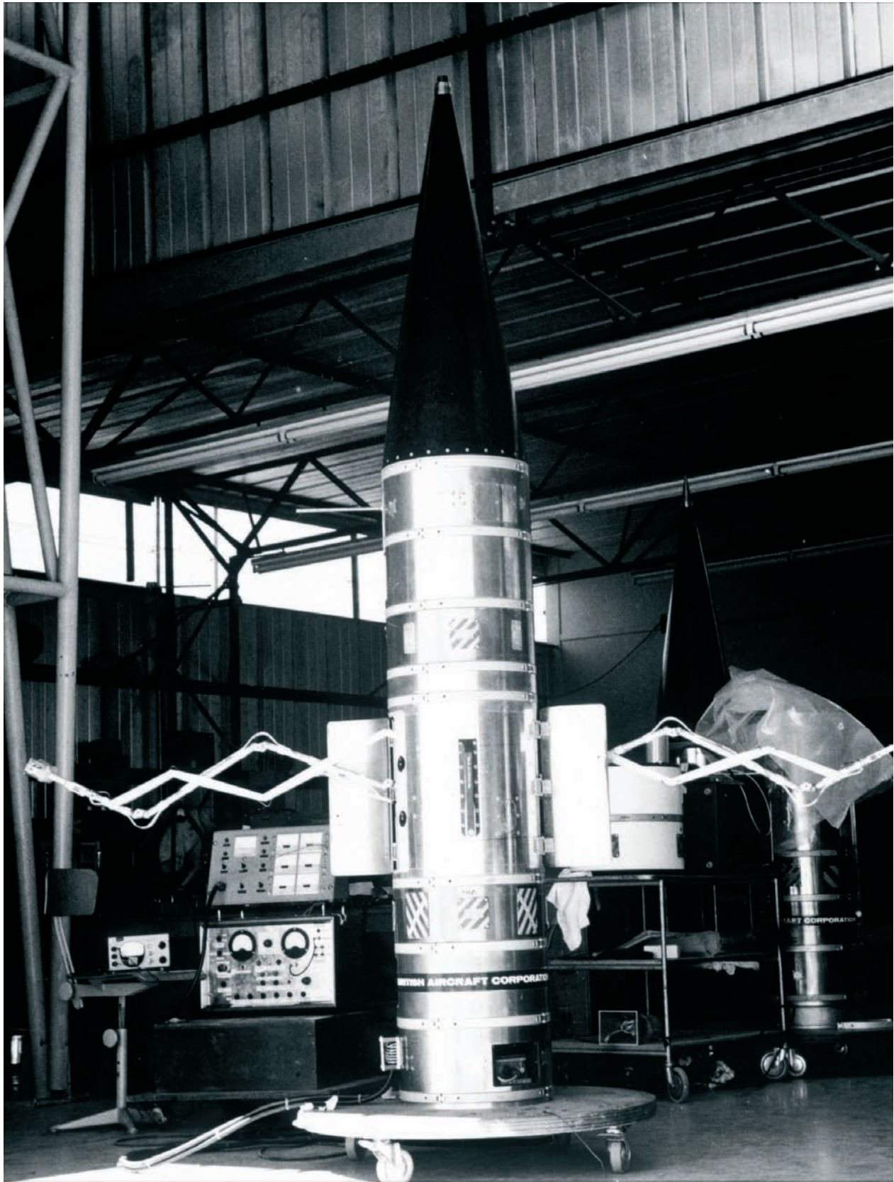
Sounding-rocket payload including impedance- and Langmuir-probe experiments, shown here with their booms deployed, being readied for launch from Sardinia in September 1967
